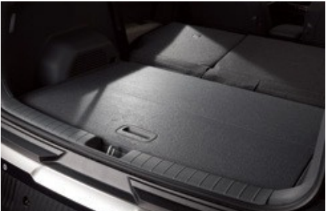
Recycled PET felt made of recycled plastics
